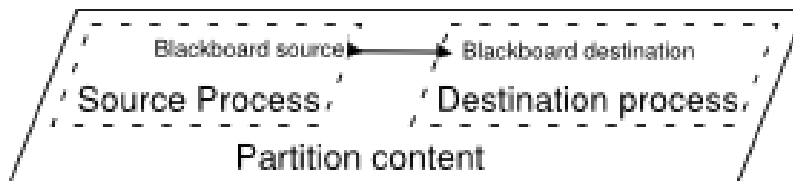
Figure 7 - Graphic representation of an ARINC 653 blackboard communication channel
